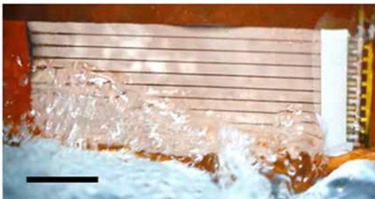
Thin-film triboelectric generator interacting with a water wave
