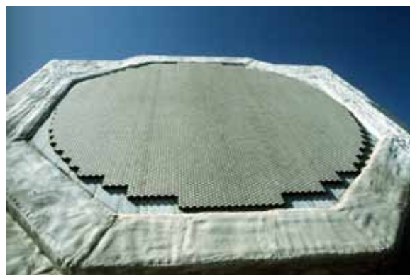
The Cobra Judy phased-array radar system on the missile range instrumentation ship USNS Observation Island. (Wikimedia Commons)
