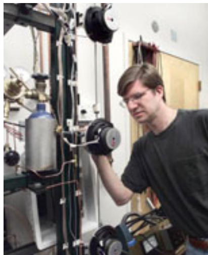
FIGURE 1: Drew Geller adjusts a speaker on a thermoacoustic separator for neon isotopes. Three of six speakers are shown, connected by the gas-separating tube.
